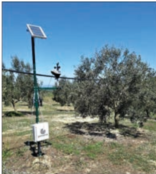
Image 3. A giasense agrometeorological station in an olive grove (by NEUROPUBLIC)
